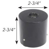
LF-AD-KNU 2" slip fitter adapter with 1/2" NPT hub in the top. Goes on 2" pipe and accepts a knuckle fixture.
